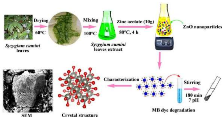
Fig 3 : Preparation scheme of ZnO Nanoparticles from Syzygium cumini leaves
